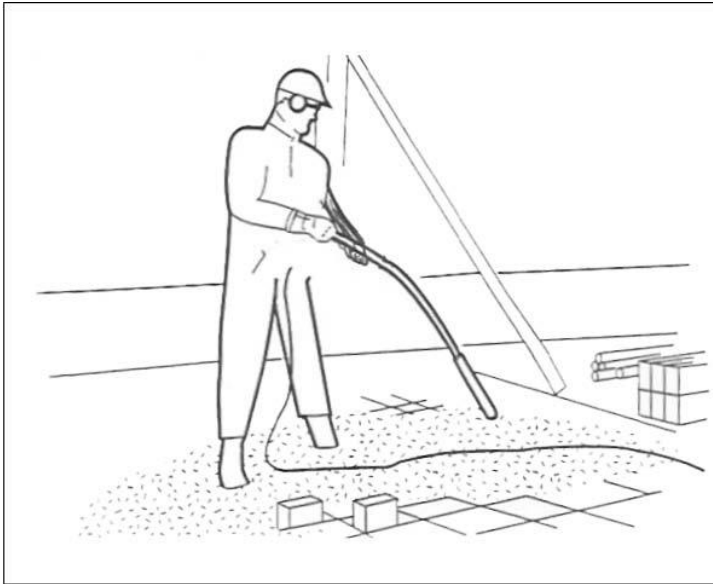
Fig. 4: Operation procedure during concrete compaction
